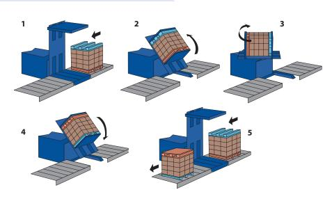
The RR can also be sited 'off-line'. The picture to the left shows how loads of boards which need turning can leave the main conveyor route, enter the RR and then return to it after inversion.
