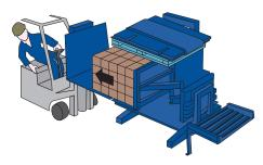
3 The clamping table rises and a second forktruck (fitted with platens and a pull-push) approaches from the side. The driver powers a moving side wall on the inverter which pushes the load onto his platens.
