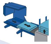
**5** The pallet is released and conveyed away to be stacked in a waiting accumulator.
