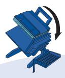
**4** He drives away to discharge his load in the container after pushing a button to return the inverter to its starting position.
