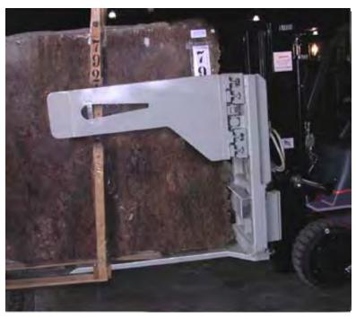
**BBJ Marble Handlers** have the capability of unloading marble and stone slabs from closed top containers.
