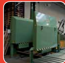
Different pallet lengths - Adaptation of the sides
